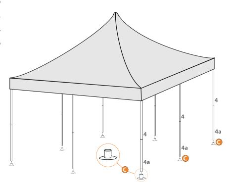
Now secure the poles with the long ground pegs. Make sure that the poles are vertical and in alignment.
